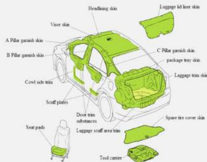
Figure 1 – Automobile parts produced from bio-based material in the Lexus CT200h. Reprinted from [12], with permission from Wiley.
