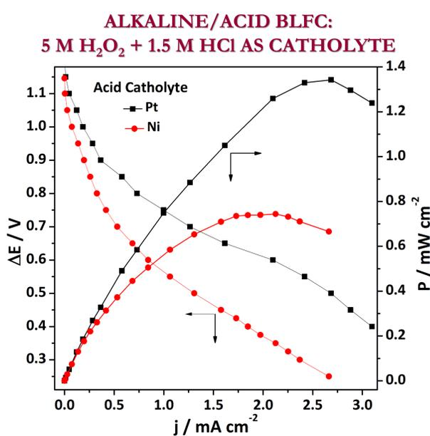
**Fig. 2:** Polarisation and power density curves for an alkaline/acid BLFC employing a Pt or Ni as anode and a Pt mesh as cathode. Catholyte was 5 M H<sub>2</sub>O<sub>2</sub> + 1.5 M HCl and black liquor was used as anolyte.
