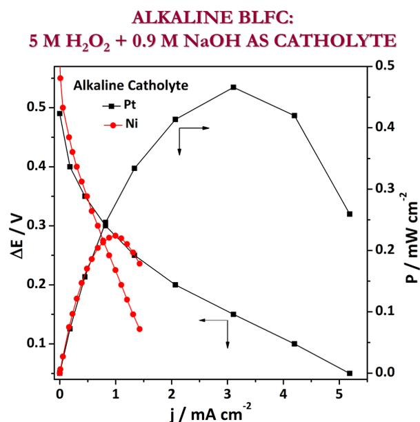
**Fig. 1:** Polarisation and power density curves for an alkaline BLFC employing a Pt or Ni as anode and a Pt mesh as cathode. Catholyte was 5 M H<sub>2</sub>O<sub>2</sub> + 0.9 M NaOH and black liquor was used as anolyte.
