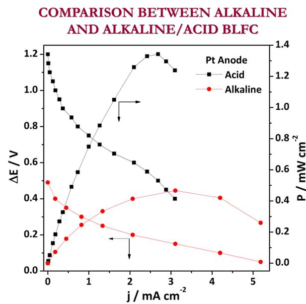
**Fig. 3:** Comparison between alkaline and alkaline/acid BLFC, employing a Pt coil as anode and a Pt mesh as cathode. Catholyte was 5 M H<sub>2</sub>O<sub>2</sub> + 0.9 M NaOH (alkaline) or 5 M H<sub>2</sub>O<sub>2</sub> + 1.5 M HCl (acid) and black liquor was used as anolyte.
